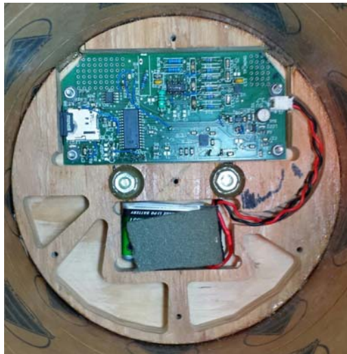
Figure 1: Looking down inside an instrumented carrier with the protective cover plate removed. An ARLISS Data Logger (Version 1) and battery are visible.
